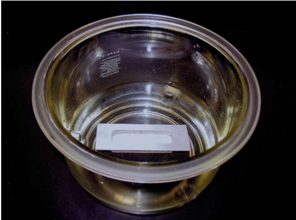
Figure 2. Water vapor cup placed in container.
